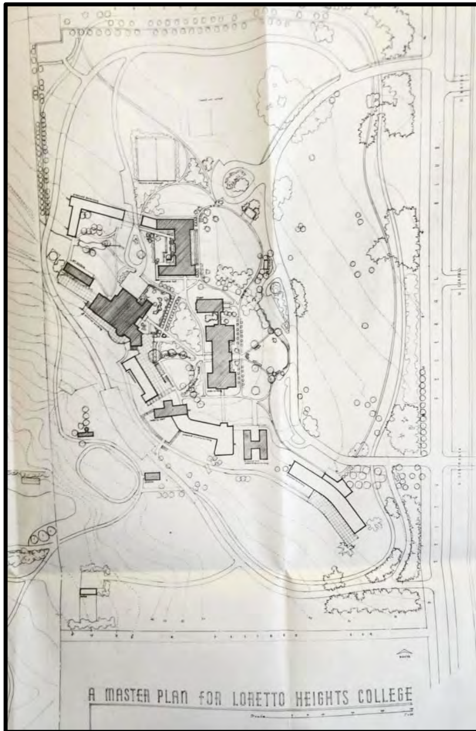
The 1950 Master Plan for Loretto Heights College, by Denver's renowned landscape architect and engineer S.R. DeBoer, recommended a semi-circular entry drive to replace the original straight drive connecting the Ad. Building to Federal Boulevard, and siting of new campus buildings to the west and southeast in order to preserve sweeping east- and west-facing views from existing buildings. Regis Archives.
